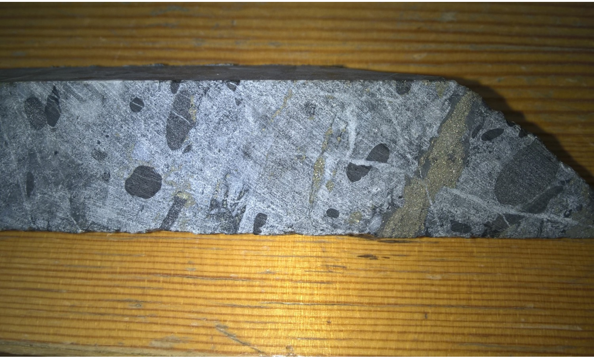
Picture 3: Drillcore from Conglomerate unit (162.20-166.45m) within ORM-1
